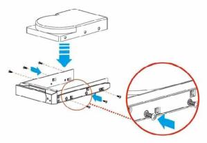
b) Place the tray with the mounted hard drive back into the case. (If the screws are not properly fastened the hard disk may be pushed towards the back of the unit and the tray handle will not open properly.)
